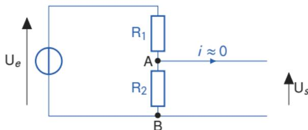
$$U_s = \frac{R_2}{R_1 + R_2} \cdot U_e$$
